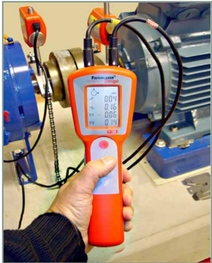
With Fixturlaser Dirigo you get the alignment result after just 3 pushed buttons.
