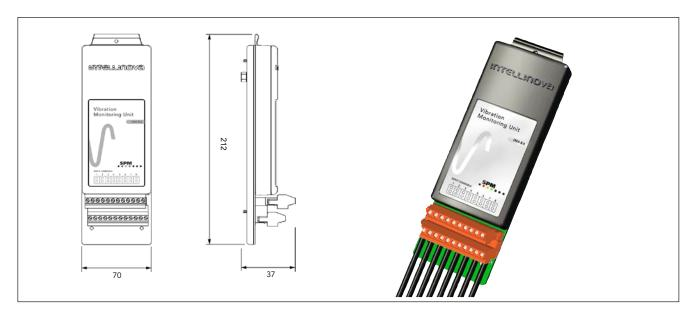
The Vibration Monitoring Unit INV80A is a part of the Intellinova System and has eight channels for continuous monitoring of vibrations. The unit is simply plugged into the socket in the Intellinova Commander Unit. Measuring time, alarm limits, alarm delay etc. are set up in Condmaster®Nova.
