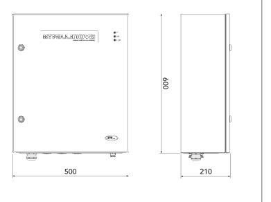
The Intellinova System Unit INS10 is comprised of an industrial enclosure, a Commander Unit, internal cabling and terminals for power supply. Monitoring units are ordered separately. The enclosure, intended for wall mounting, is robust and sealed for use in harsh environments.
