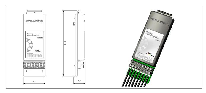
The Bearing Monitoring Unit is a part of the Intellinova System and has eight channels for continuous monitoring of bearing condition. It measures shock pulses according to the True SPM method and supports SPM Spectrum. The unit is simply plugged into the socket in the Intellinova Commander Unit. Measuring methods, measuring time, alarm limits, alarm delay etc. are set up in Condmaster®Nova.
