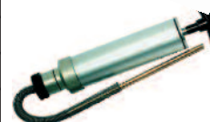
F7828000 Manual Pump for Smoke Index Measurement
